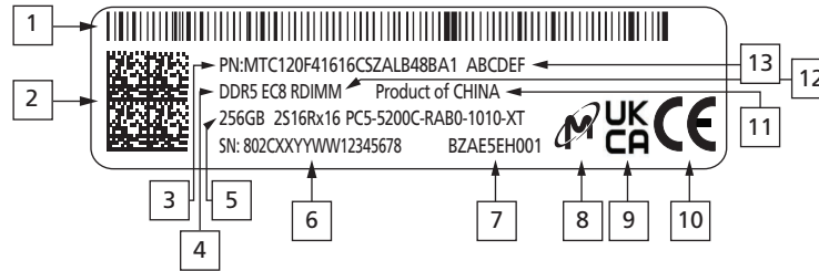
Figure 4: DDR5 LRDIMM, RDIMM, UDIMM and SODIMM DRAM Module Label Content
