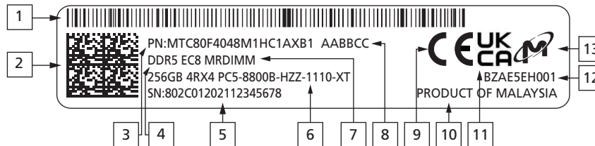
Figure 5: DDR5 MRDIMM DRAM Module Label Content
